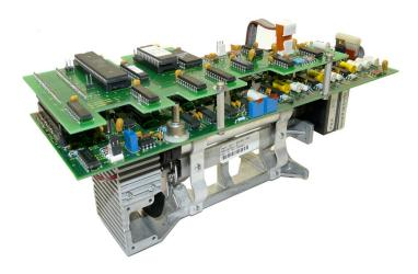
The 6230 and 6231 provide fully corrected HC, CO, CO2 and O2 gas concentrations in digital form via an industry standard RS232 serial communications interface.
