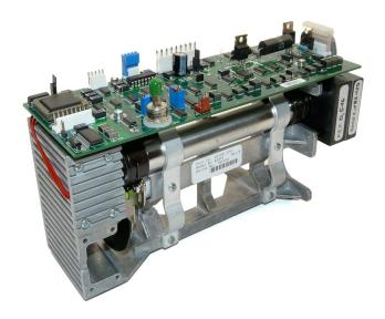
The 6231A and 6241A are the direct predecessor of the famos 62XX series. They are based on the design architecture of the world's most field proven and reliable digital IR gas analyzer bench with over 160,000 installations world-wide, pioneered by Andros. These new models now incorporates new surface mount technology (SMT) with a highly powered microprocessor for even greater performance.
